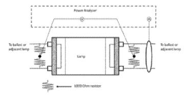
Figure 1: Programmed- and Rapid-Start Ballast Instrumentation Scrap
