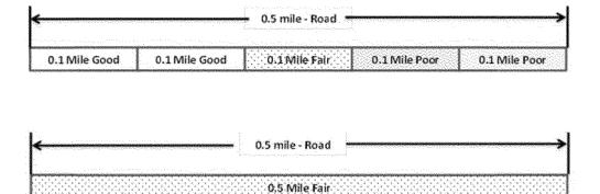
Figure 8 - A <sup>1</sup>/<sub>2</sub>-mile road is measured at (a) 0.1-mile section and (b) the same road is
