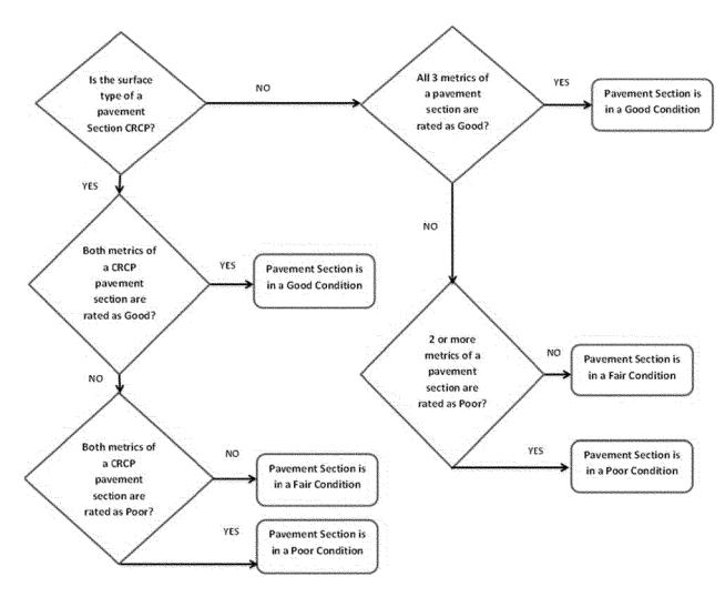
Legend: CRCP=Continuously Reinforced Concrete Pavement
