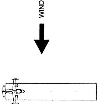
PRIOR TO TOUCHDOWN, THE UPWIND WING IS LOWERED AND SMOOTHLY MODULATED. OPPOSITE RUDDER IS APPLIED SO THAT AIRCRAFT PATH CONTINUES DOWN RUNWAY CENTERLINE. THE AIRCRAFT SHOULD NOT BE ALLOWED TO DEVELOP ANY TENDENCY TO DRIFT DOWNWIND.
