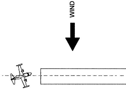
AIRCRAFT WILL BE FLOWN DOWN AN EXTENSION OF THE RUNWAY CENTER LINE WITH DRIFT CORRECTION ESTABLISHED SUFFICIENTLY IN ADVANCE TO PERMIT CENTER LINE TO BE FLOWN WITH ONLY MINOR COORDINATED CORRECTIONS
