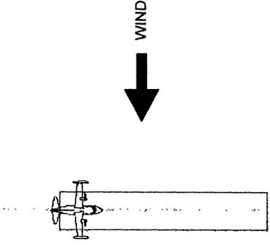
PRIOR TO TOUCHDOWN, THE UPWIND WING IS LOWERED AND SMOOTHLY MODULATED. OPPOSITE RUDDER IS APPLIED SO THAT AIRCRAFT PATH CONTINUES DOWN RUNWAY CENTERLINE. THE AIRCRAFT SHOULD NOT BE ALLOWED TO DEVELOP ANY TENDENCY TO DRIFT DOWNWIND.
