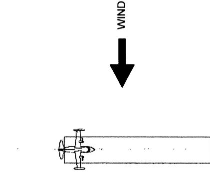
PRIOR TO TOUCHDOWN, THE UPWIND WING IS LOWERED AND SMOOTHLY MODULATED. OPPOSITE RUDDER IS APPLIED SO THAT AIRCRAFT PATH CONTINUES DOWN RUNWAY CENTERLINE. THE AIRCRAFT SHOULD NOT BE ALLOWED TO DEVELOP ANY TENDENCY TO DRIFT DOWNWIND.
