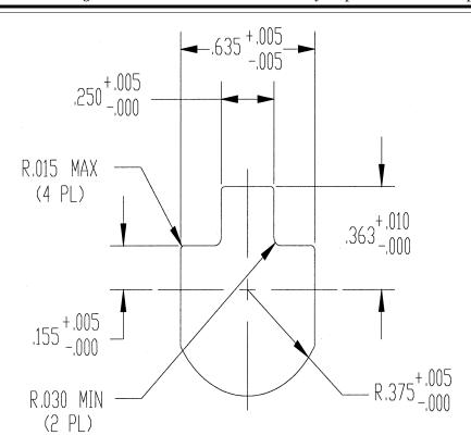
Figure 14. Mounting Hole, PSIN 0910 Customer Lock
